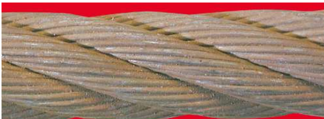
a. Beginning of surface oxidation, can be wiped clean, Superficial — rating: 0% towards discard
