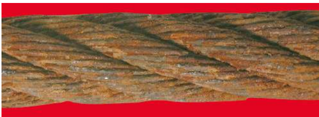
c. Surface of wire now greatly affected by oxidation - rating: 60% towards discard
