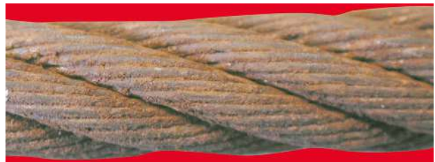
b. Wires rough to touch, general surface oxidation — rating: 20% towards discard
