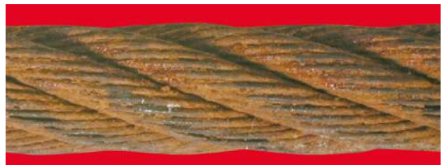
d. Surface heavily pitted and wires quite slack, gaps between wires — discard immediately
