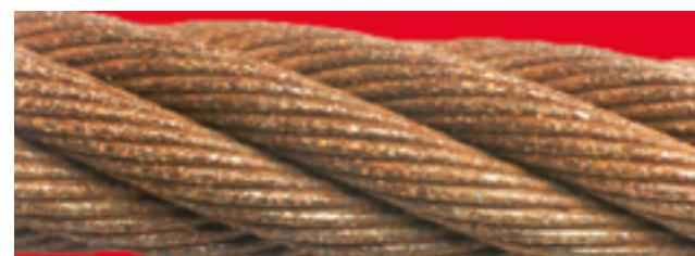
i. Enlargement of External corrosion
