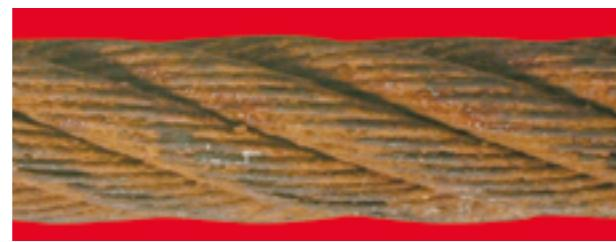
d. Surface heavily pitted and wires quite slack, gaps between wires — discard immediately
