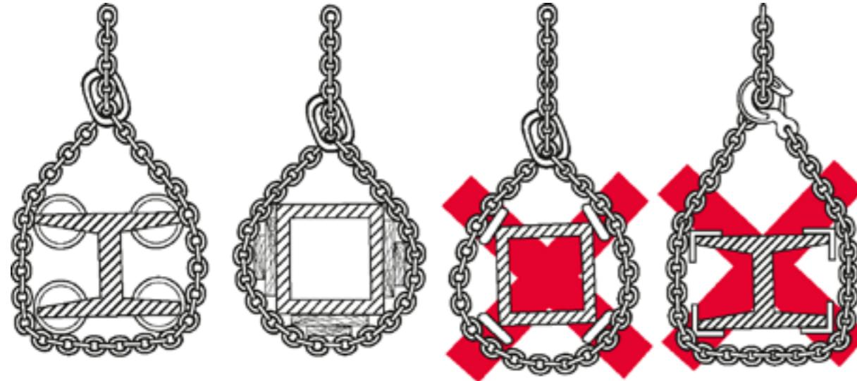
If chains are guided over edges without proper protection, their load capacity is significantly reduced and safe usage can no longer be guaranteed. Where chain has to be looped around beams or other round - shaped loads, the diameter should be at least twice or 3 times the chain pitch. For smaller diameters, the load capacity of the chains must be reduced by 50%.
