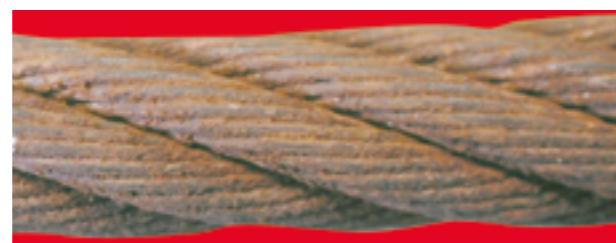
b. Wires rough to touch, general surface oxidation — rating: 20% towards discard
