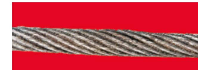
l. Local increase in rope diameter due to core distortion
