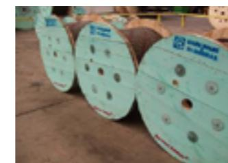
Steel wire ropes should be stored in closed, dry and cool environment. Direct contact with the ground must be cut. If open storage is to be done, suitable packaging should be made to prevent rusting due to wet, moisture and humidity.
